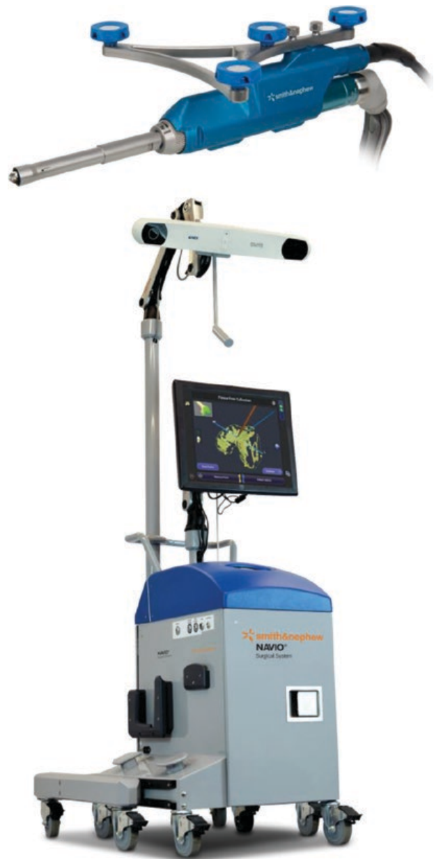
Fig. 13.2 The Navio handheld image-free robotic sculpting device with handpiece
